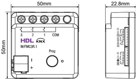
Figure 2. Dimensions - Front View Figure 3. Dimensions - Side View
