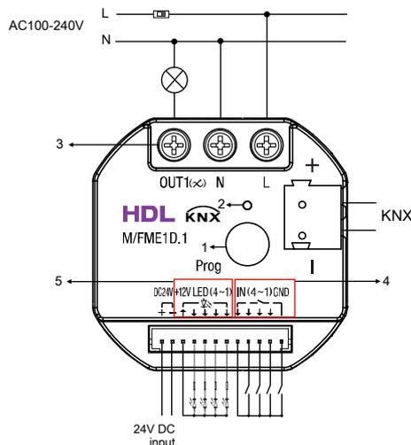
Figure 4. Wiring
