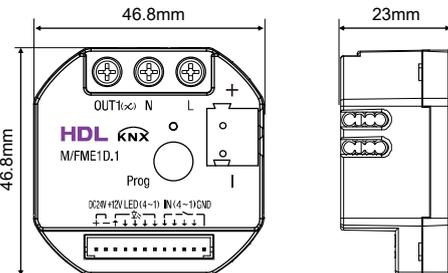
Figure 2. Dimensions - Front View Figure 3. Dimensions - Side View
