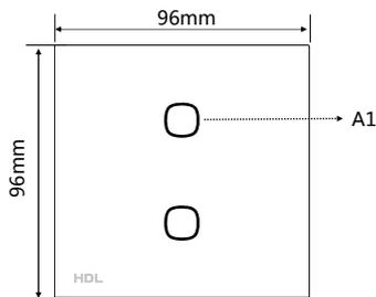
Figure 5. Dimensions - Front View
