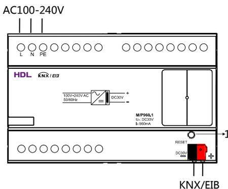
Figure 4. Wiring
